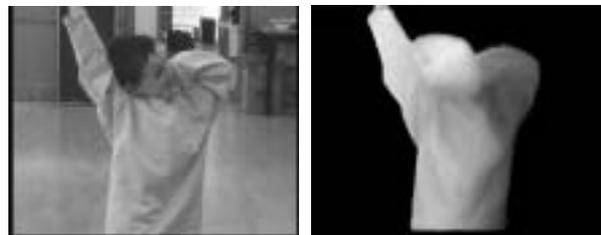
Figure 5. A color frame and its corresponding depth frame. Background objects are outside the depth measurement window.
