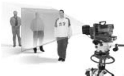
Figure 4. Dynamically setting the depth window, controls the volume measured by the camera.
