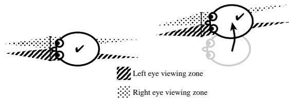
Figure 4: an alternative mechanism for head-tracking: only two zones are produced, but the image display mechanism can control where those two views are in space.
