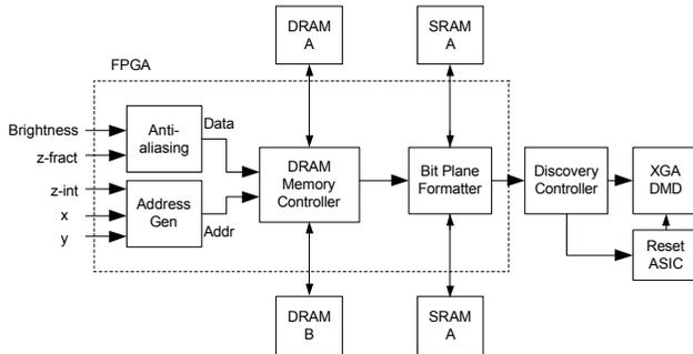
Figure 3. Block diagram of a DepthCube color channel.
