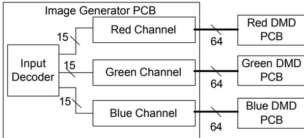
Figure 2. Block diagram of DepthCube Electronics.
