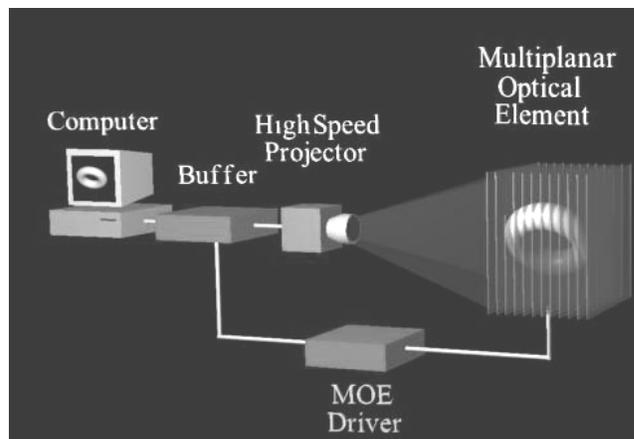
Figure 1 Schematic diagram of the DepthCube™ 3D Display System.
