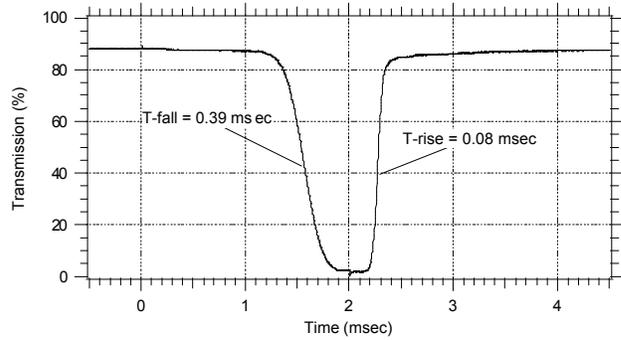
Figure 4. Transmission vs. time of PSCT shutter.
