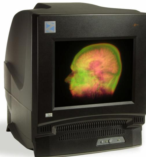
**Figure 5. Photograph of a commercial DepthCube 3D Display.**
