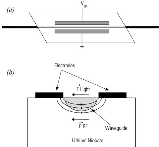
Fig. 7: Integrated-optic phase modulator (a) top view, and (b) side view
