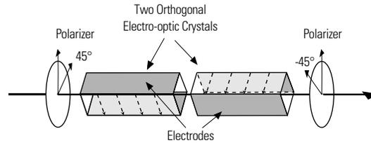
Fig. 3: Thermal bias drift can be passively compensated using two crystals oriented orthogonally with respect to each other. In the case shown above, the crystals are mounted at  $45^\circ$ . Thus, the input polarization is vertical. The applied field is reversed in the second crystal. In this manner, the thermal birefringence is compensated but the desired birefringence is doubled.
