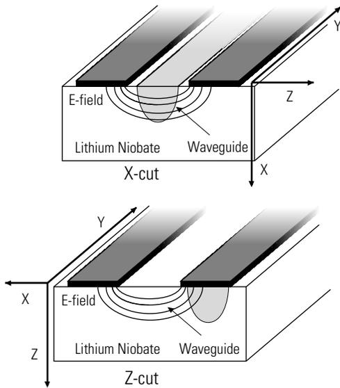
Fig. 10: Geometry of  $\text{LiNbO}_3$  modulators.
