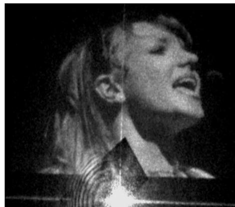
**Figure 5 - Example replay field produced using 1280 x 1024 binary holograms using OSPR ( $N = 24$ )**
