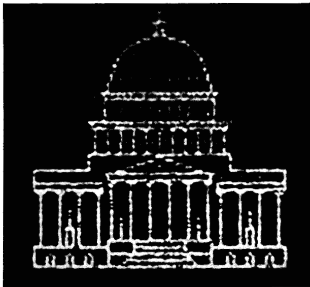
Figure 9 Image reconstructed from a binary hologram with diffuser noise reduced.
