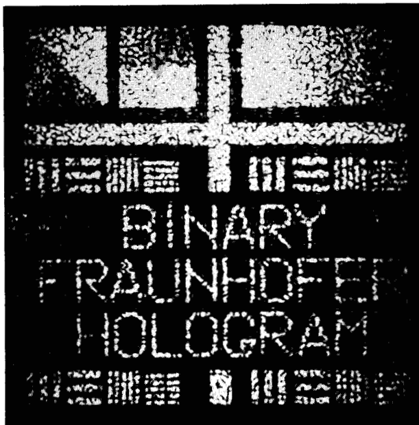
Figure 8 Image reconstructed from a binary hologram showing resolution, grey tones, and noise from a simulated diffuser.
