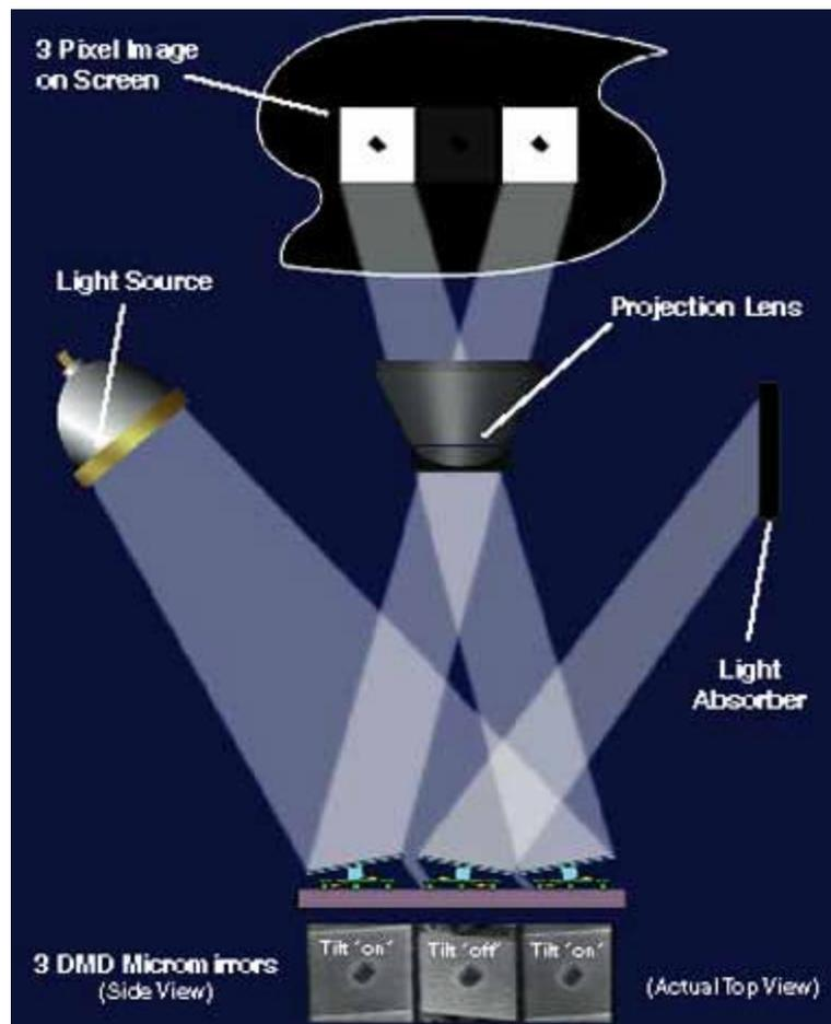
Three mirrors efficiently reflect light to project a digital image. Incoming light hits the three mirror pixels. The two outer mirrors that are turned on reflect the light through the projection lens and onto the screen.
