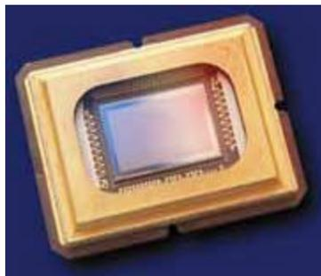
An 848 x 600 Digital Micromirror Device. The central, reflective portion of the device consists of 508,800 tiny, tiltable mirrors. A glass window seals and protects the mirrors.
