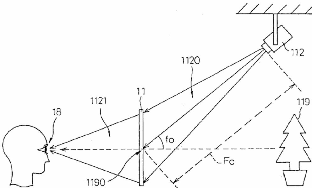
**Figure 2. Diffraction of Light by Holographic Screen (11)**
