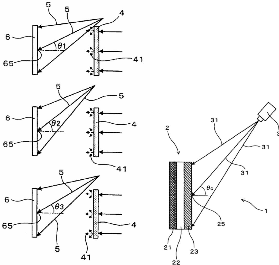
**Figure 5 Three Wavelength Holographic Projection Screen Recording Setup**
