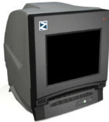
**Figure 7.** Actuality Systems Perspecta<sup>®</sup> (left) and VIZTA<sup>3D</sup> Z 20|20<sup>TM</sup> (right) volumetric displays. Both use 3 DMDs to create 3D images viewed without glasses or headsets.
