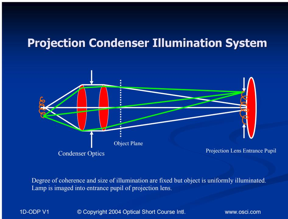
Figure 3. Projection Condenser Illumination System Layout
