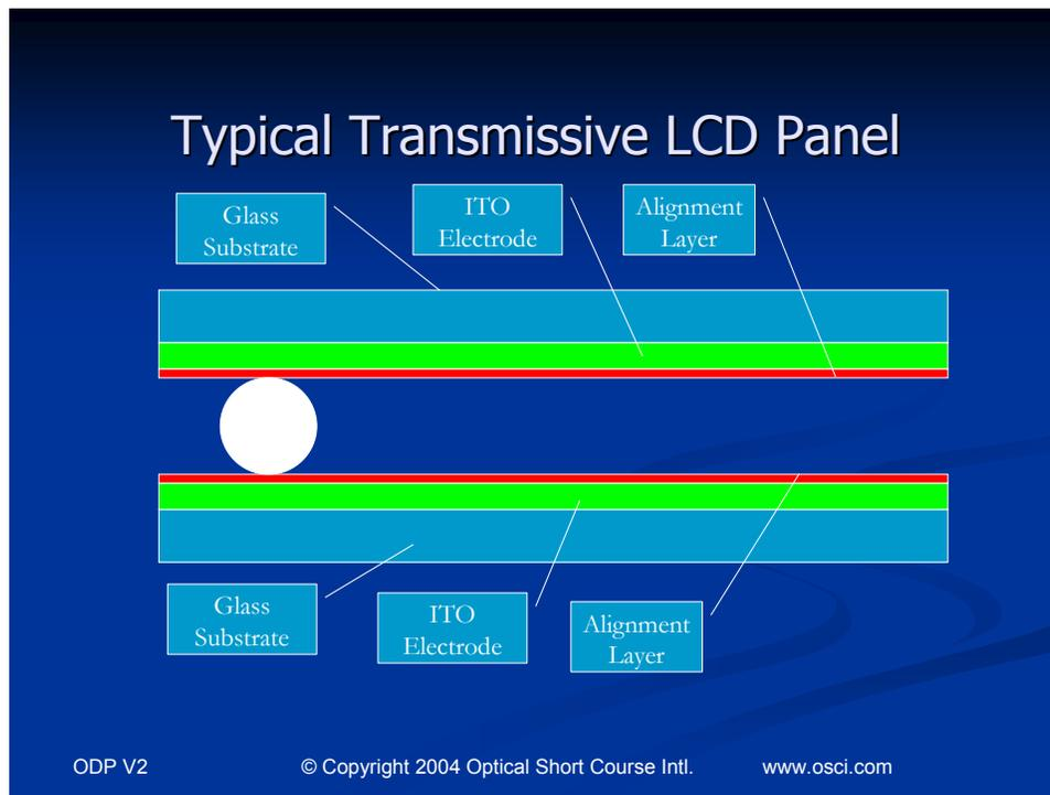
Figure 1. LCD Panel Cross Section View
