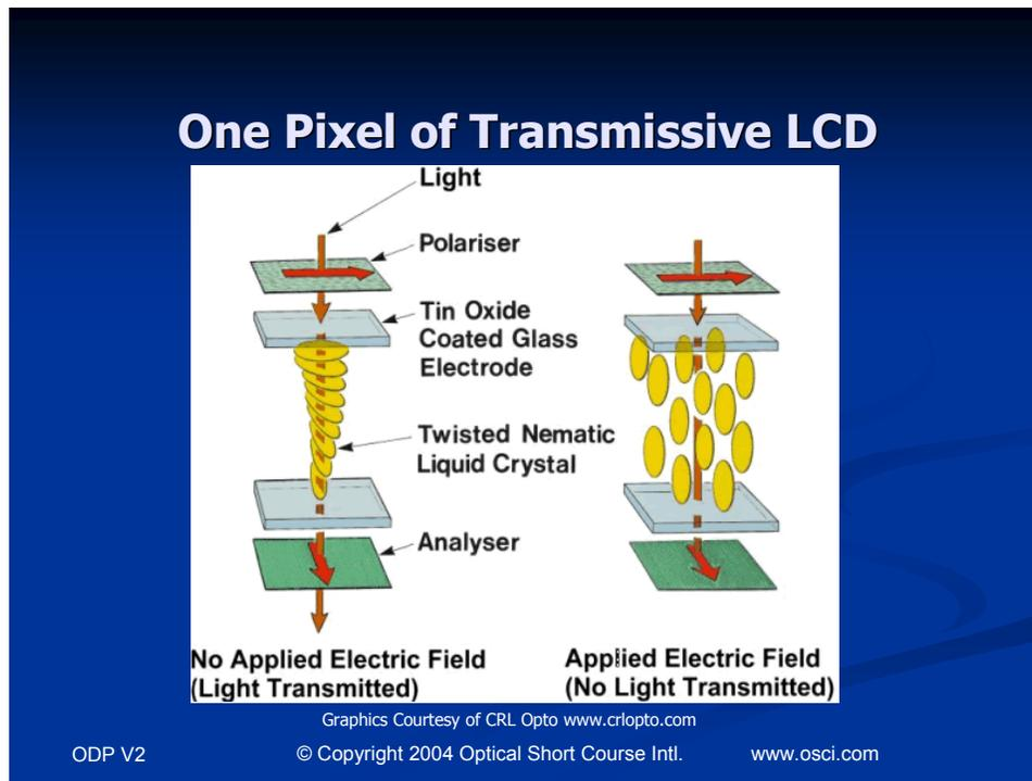
Figure 4. LCD Panel Principle of Operation
