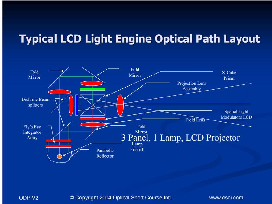
Figure 6. Parallel Color System – LCD Light Engine
