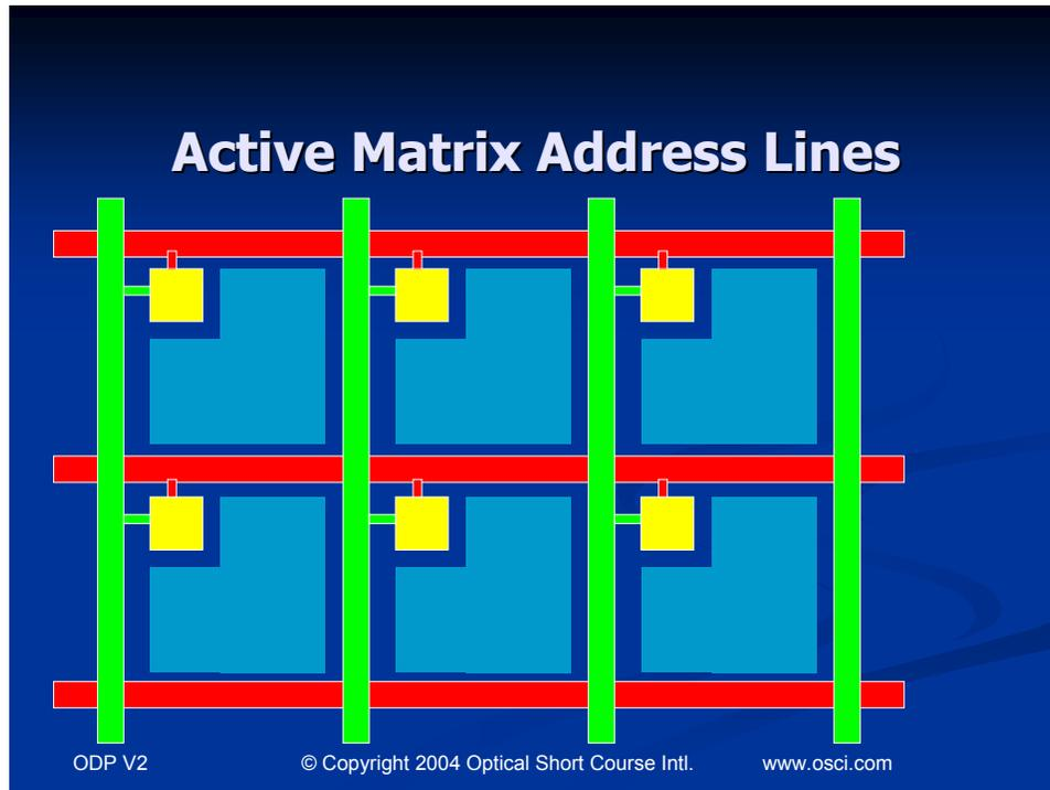
Figure 2. Active Matrix Address Lines Create Screen Door Effect
