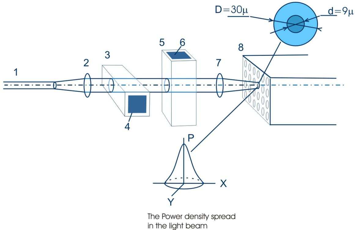
**1** - fiber; **2** - input forming optical system; **3** - 1<sup>st</sup> AO crystal (x-dimension); **4,6** - transducers; **5** - 2<sup>nd</sup> AO crystal (y-dimension) **7** - output forming optical system; **8** - output matrix of the fibers
