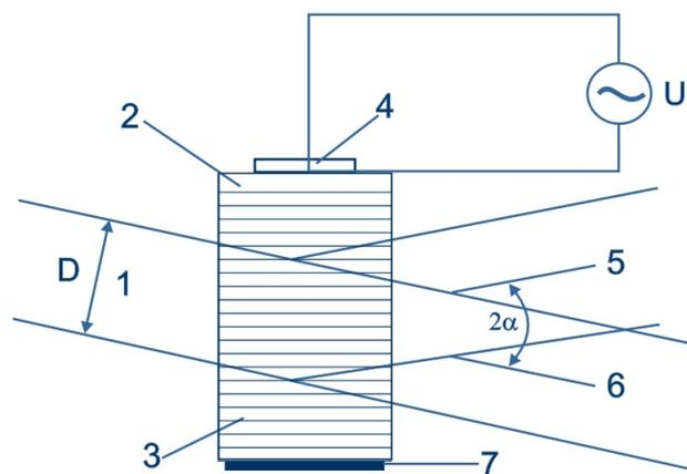
1 - input beam; 2 - acousto-optic crystal; 3 - regular structure created with ultrasonic wave; 4 - transducer; 5 - deflected beam; 6 - output beam passed without transformation (zero order); 7 - ultrasound absorber
