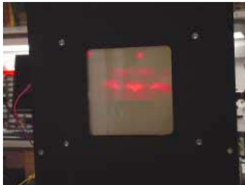
FIGURE 2. An eight-layer liquid-crystal volumetric display with layers separated by 4.6 mm has a 15-cm viewable size. The fuzziness of this projected image is more an effect of the sheets rather than a lack of inherent resolution of the DMD.
