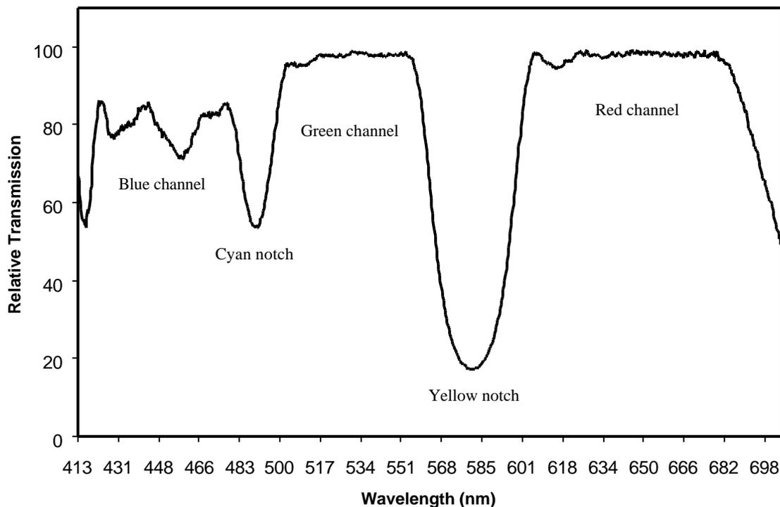
Figure 7: Typical yellow notch filter<sup>4</sup> used to increase color gamut for DLP cinema projectors.
