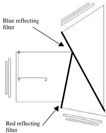
Figure 4: Prism design for DLP projection showing the red and blue dichroic filters
