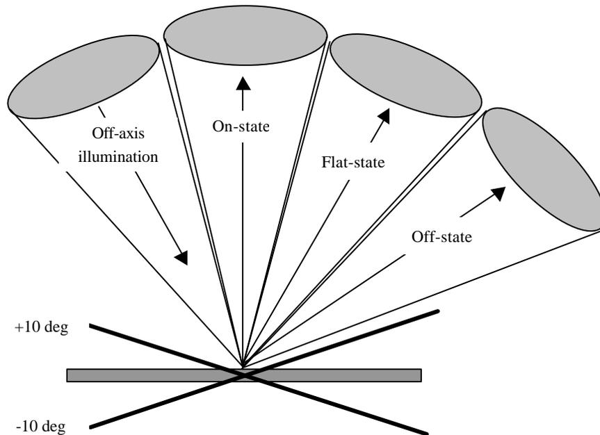
Figure 2: Off-axis illumination of DMD is used to separate on-state, flat-state and off-state.
