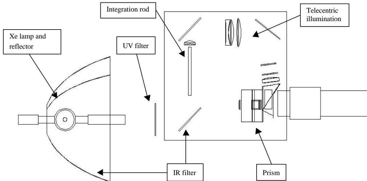
Figure 3: Optical layout of digital cinema projector showing the illumination optics and the various filters for UV, IR and color notching
