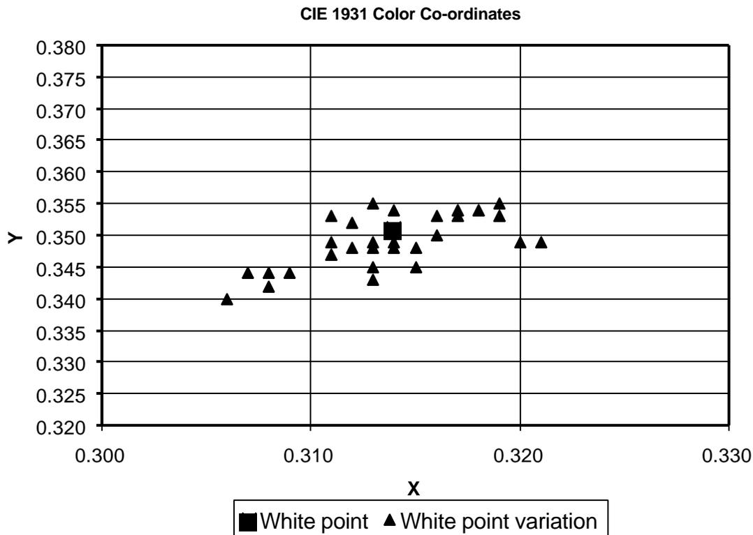
Figure 8: Color chart showing the variation that occurs in the white point as a result of oscillations in the transmission of the yellow notch filter.
