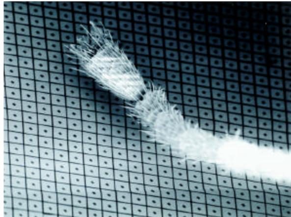
Figure 1: Picture of DMD showing micro-mirrors relative to an ant leg (courtesy of Texas Instruments Incorporated).
