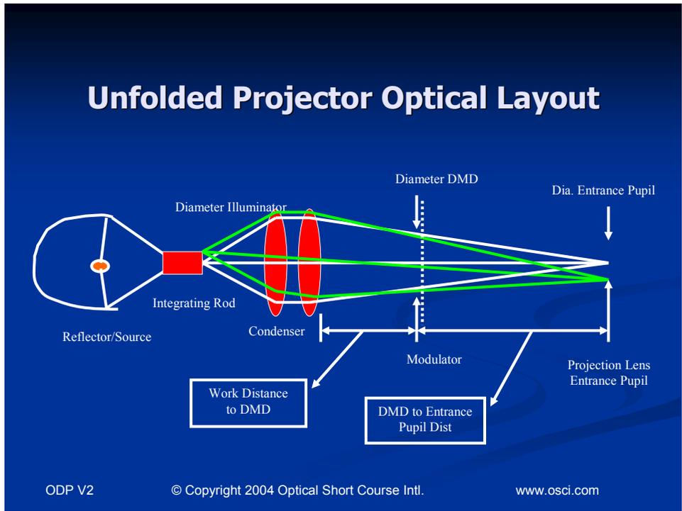
Figure 3. Digital Projector Light Engine Illumination System Layout
