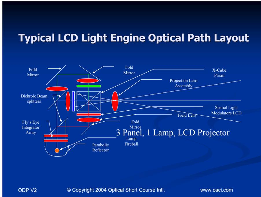
Figure 2. Parallel Color System – LCD Light Engine
