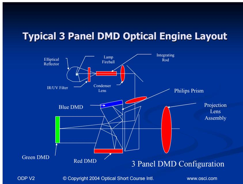
Figure 3. Parallel Color System – 3 Panel DMD Light Engine
