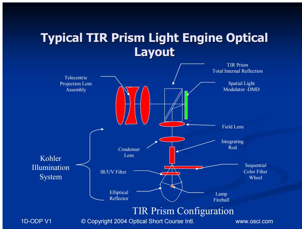
Figure 4. Single Panel DMD Light Engine Layout
