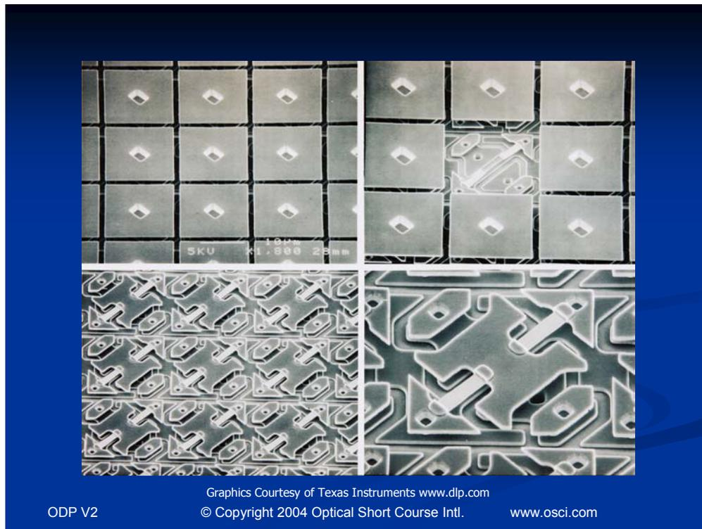
Figure 2. SEM of DMD™ Mirrors, Yoke, Torsional Flexure, Address Electrodes
