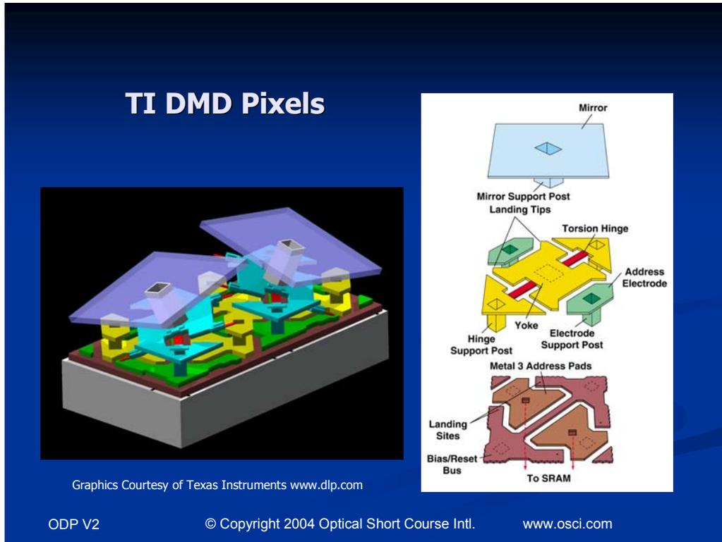
Figure 1. DMD™ Panel Cross Section View
