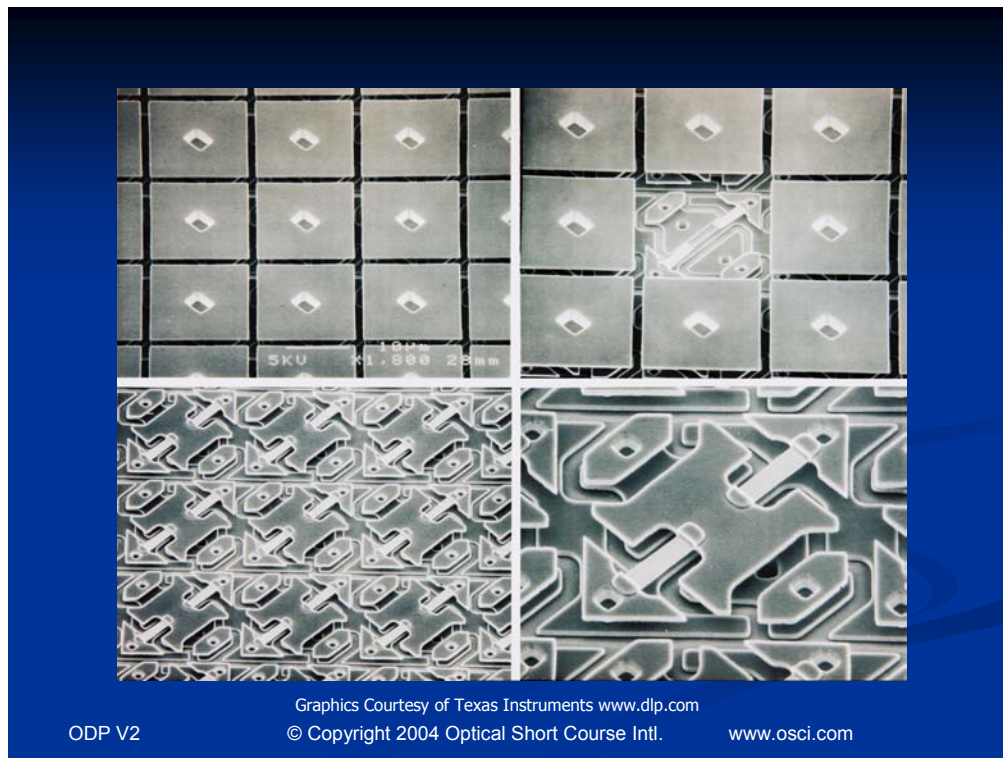
Figure 2. SEM of DMD™ Mirrors, Yoke, Torsional Flexure, Address Electrodes Graphics Courtesy of Texas Instruments http://www.dlp.com From OSCI's Optics of Digital Projectors DVD Course http://www.oscintl.com/prod01.htm
