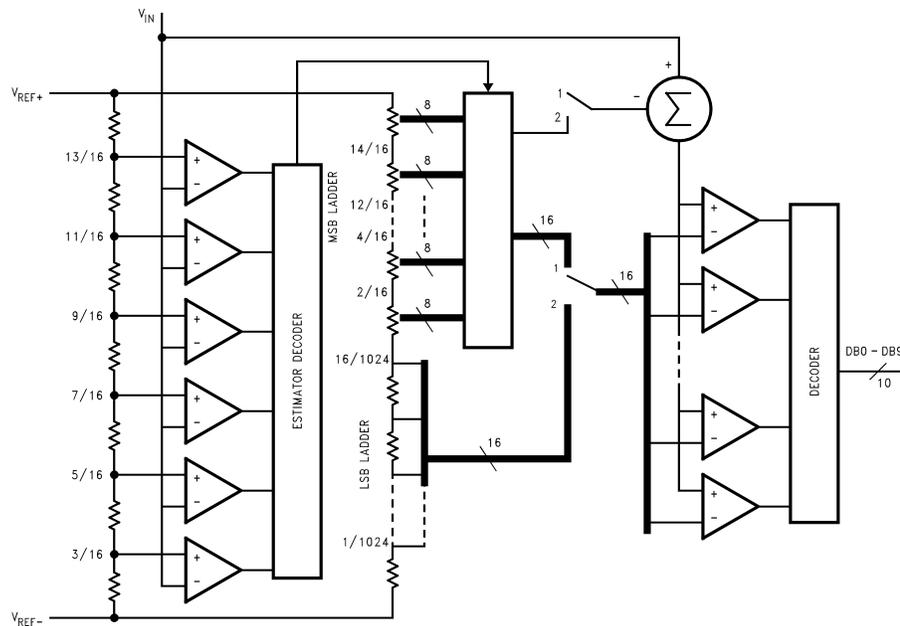
FIGURE 3. Block Diagram of the Multistep Converter Architecture
