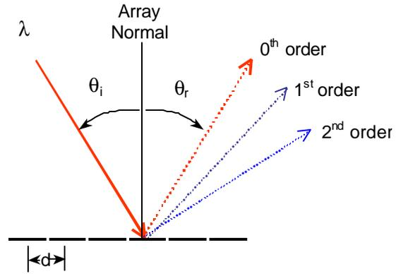
Figure 2. Incident light hitting a grating (SBG) with periodicity  $d$  and mirror-pixels inactive or “parked” at 0 degrees. In this example most of the incident light undergoes specular reflection and gets spread out over a number of low-irradiance orders.
