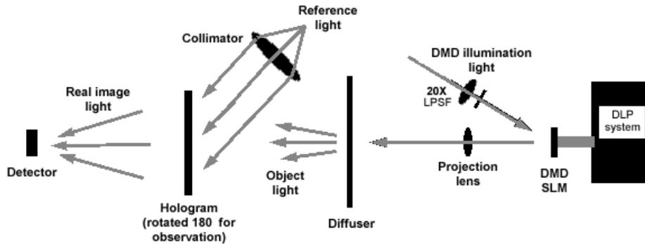
Figure 9. DMD holographic recording and projection setup (Not shown: LCD in rear-lit configuration)
