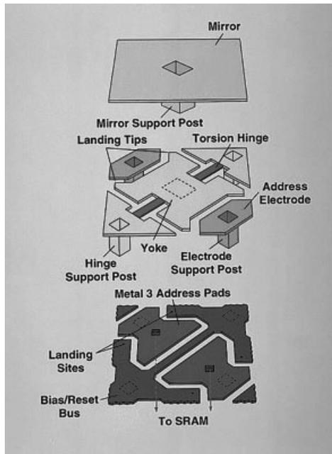
Figure 1. DMD microstructure
