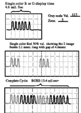
Figure 5. Projector timing and sequence
