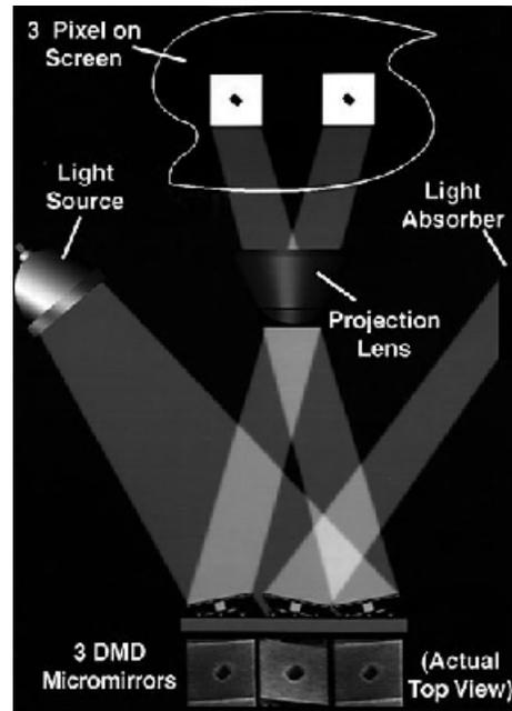
Figure 2. DMD optical switching method
