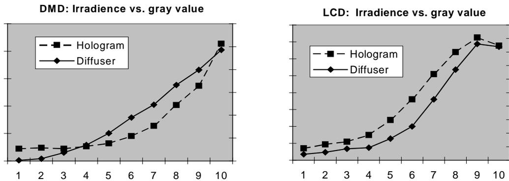
Figure 10. Irradiance measured at diffuser and projected real image plane for ten grayscale steps for DMD and LCD
