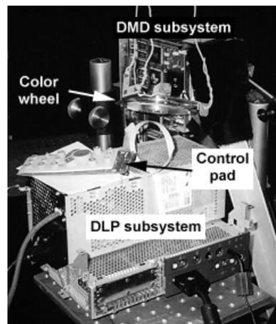
Figure 8. DLP components (viewed from backside)
