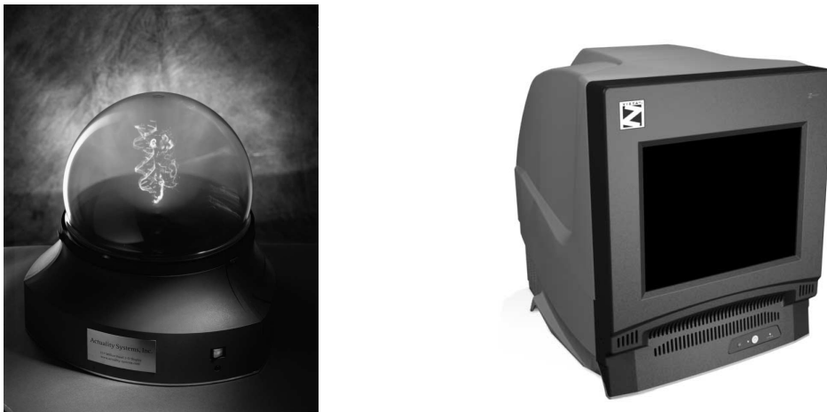
Figure 7. Actuality Systems Perspecta ® (left) and VIZTA 3D Z 20|20 ™ (right) volumetric displays. Both use 3 DMDs to create 3D images viewed without glasses or headsets.
