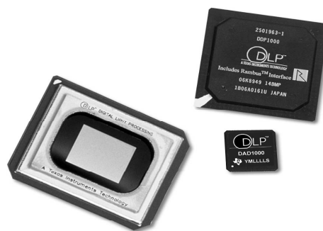
Figure 16. Discovery 1000 chipset with 0.7 XGA DDR DMD, digital controller, and analog mirror reset driver
