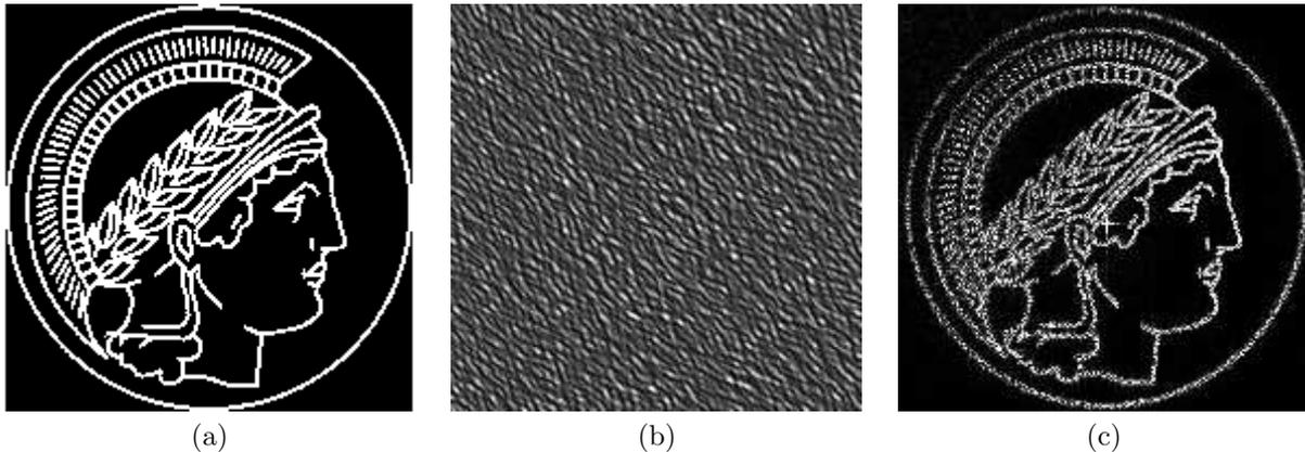
**Figure 3.** input image (a), hologram (b) and reconstruction (c) of an emblem of the greek goddess Minerva. The hologram is constructed with 8192 sample points in 5.8 s, and has a size of  $512^2$  image points. It is reconstructed using the Fresnel approximation.
