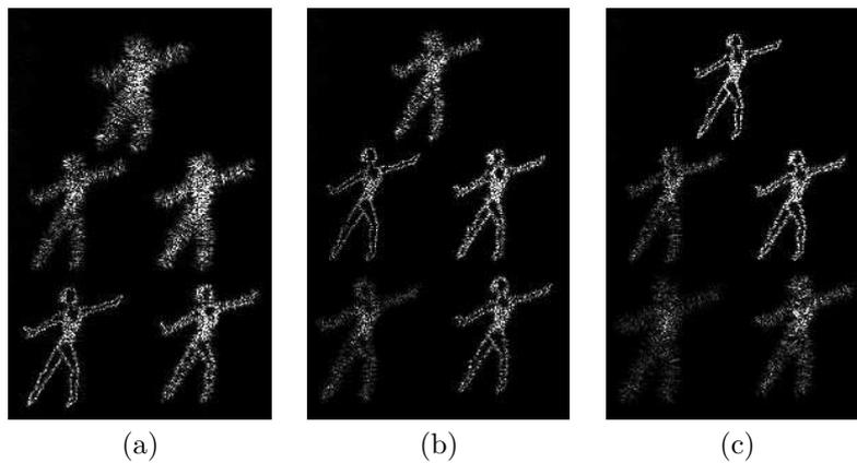
**Figure 4.** Fresnel approximated reconstructed view of an hologram with 5 dancers at different distances. Nearest to the hologram plane is the dancer in the lower-left corner at a distance of 1.26 cm, farthestmost is the upper dancer at 1.64 cm. The hologram is constructed with 4096 sample points in an off-axis geometry. Reconstruction: (a) nearest dancer in focus, (b) middle-left dancer in focus and (c) upper dancer in focus.
