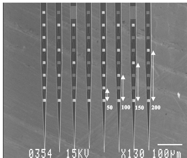
**Figure 7.** SEM picture of selectively opened electrode windows in  $\text{Si}_3\text{N}_4$  layer on probe shafts. The site distance varies from  $50 \mu\text{m}$  to  $200 \mu\text{m}$ . Bright squares are opened windows.
