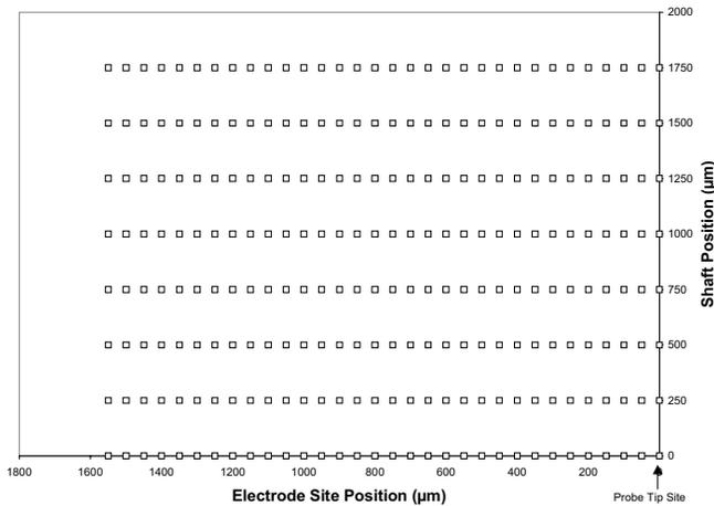
Figure 2. Proposed snap grid for on-demand probes.
