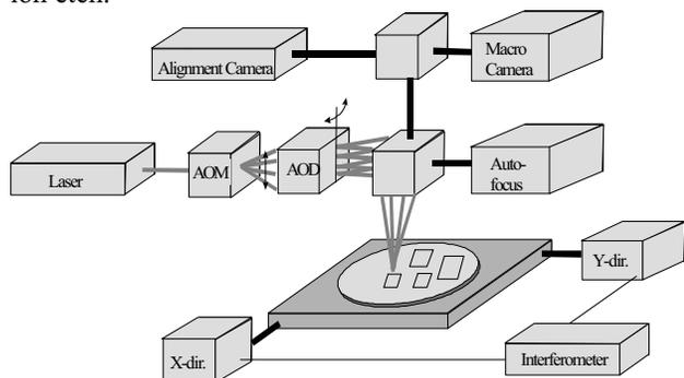
**Figure 6.** Schematic picture of the DWL principle.
