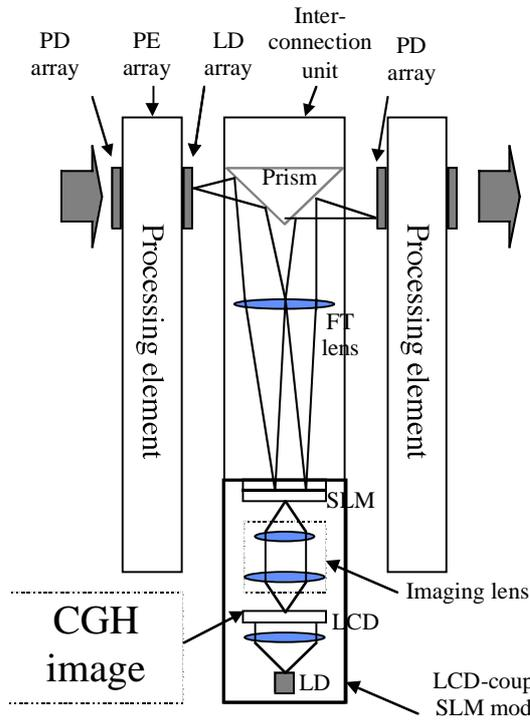
Fig. 2. Implementation of two layers of the pipeline.
