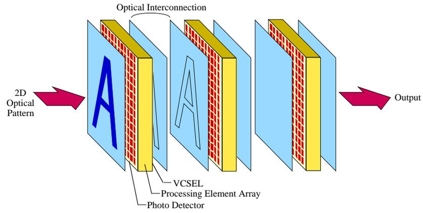
Fig. 1. Conceptual drawing of free-space interconnected pipelined architecture.
