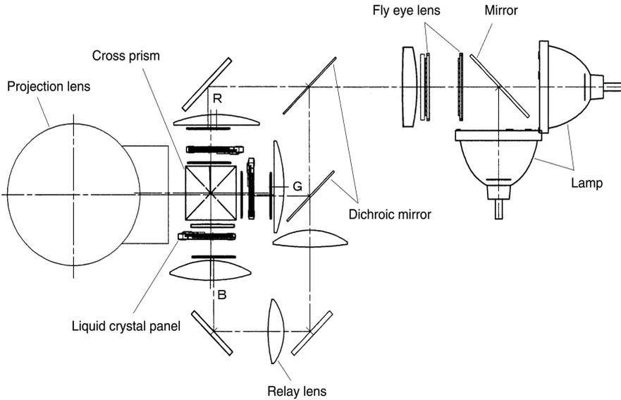
Fig. 1 CGS TFT LCD projection optical engine.
