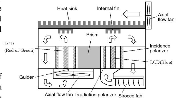
Fig. 3 Closed cooling system.
