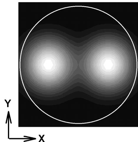
Fig. 5 Intensity distribution of the light source image in the pupil.
