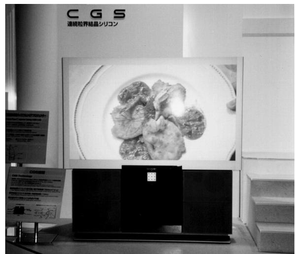
Photo 1 60" LCD rear projection HDTV.
