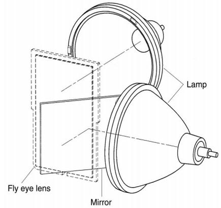
Fig. 2 Lamp system of optical engine.
