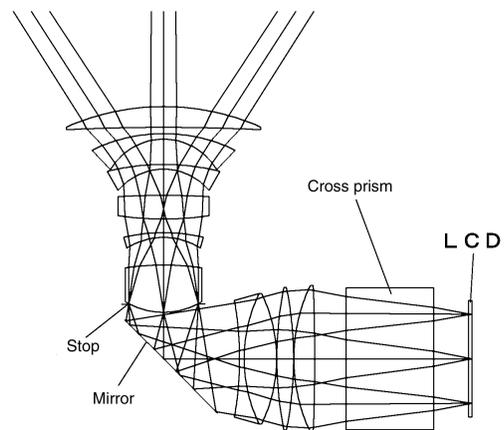
Fig. 4 Optical path of projection lens.
