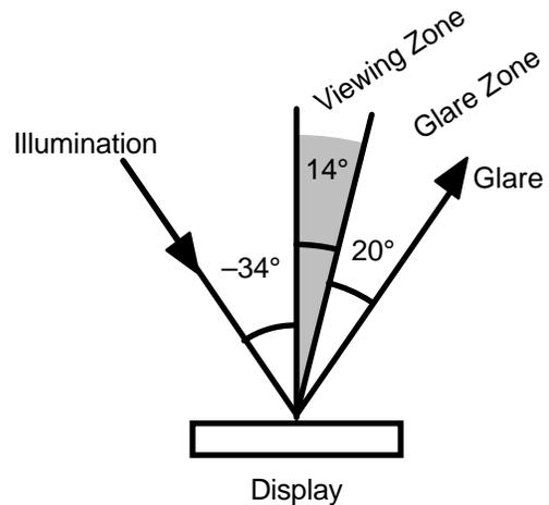
**Figure 4.** For illumination at  $-34^\circ$  the viewing zone is confined to a small range of angles near the display normal, which forms one boundary. The other boundary is the glare zone which is a range of angles ( $20^\circ$ ) over which glare interferes with viewing.
