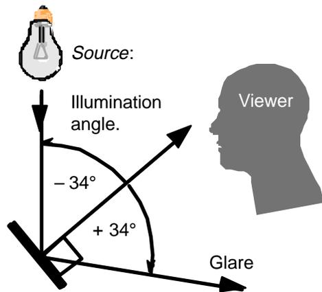
**Figure 3.** Optimum design angle for incidence of source illumination on the display is 34° as determined by tests based on variations in overhead lighting and comfortable head positions. It is assumed that the preferred viewing angle is perpendicular to the display. Illumination angles are measured from the normal. Source-normal angle is defined to be negative.
