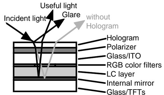
**Figure 2.** Proposed stackup of color reflective LCD with a transmission hologram on the top. Light path shown as black lines. Gray line indicates light path without hologram. The hologram both steers and scatters the incoming light.
