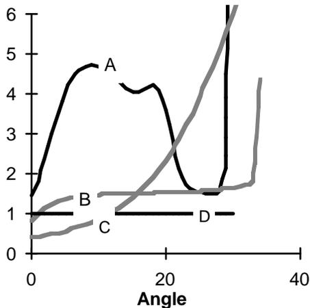
**Figure 5.** Measured luminance gain of a transmission hologram (A). The hologram is affixed to a specular reflector for the measurement. Source is at  $-34^\circ$ . For comparison, a Polaroid LIFT green reflection hologram (B) is included along with a typical metallic reflector for LCDs (C). The luminance gain is relative to the white, diffuse, reflectance standard, Spectralon [D].
