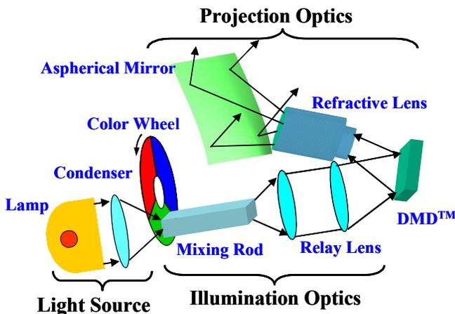
**Figure 5. Outline layout of the optical engine**
