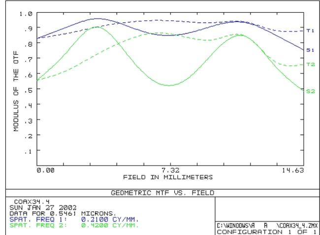
**Figure 4. MTF vs. field characteristics on the screen side. Calculation is done at spatial frequencies of 0.21 and 0.42 mm<sup>-1</sup>, wavelength of 546.1nm. Note that field between 0mm and 2.1mm is not used. Due to the small color aberration as shown in Fig. 3, little degradation occurs even if multiple wavelength MTF is considered.**
