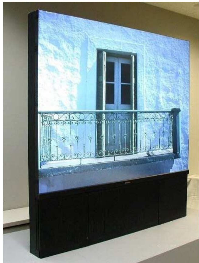
Photo 1. External appearance and displayed image of the prototype rear projector
