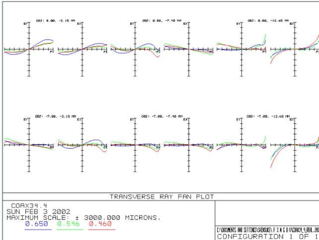
**Figure 3. Transverse ray aberrations on the screen side. Each EX/EY graph shows aberrations at 6 grid points in the right half image area of 60-in. diagonal. Calculation wavelengths are 650, 546 and 460nm. Nearly negligible lateral color aberrations as compared to a pixel pitch of 1.2mm are seen.**
