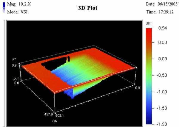
Grayscale ramp in photoresist
