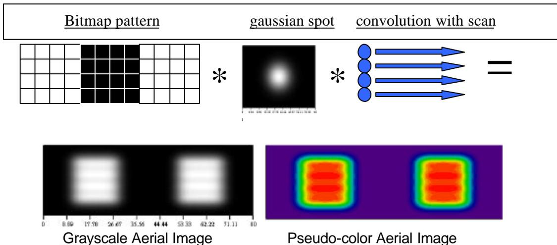
Note that the nature of the raster imaging process causes asymmetry in the maximum spatial frequency for horizontal and vertical lines. This is caused by the additional convolution in the fast-scan direction. As long as the pixel spacing and spot size are sufficiently small relative to the feature size (i.e. many pixels per feature), this effect is not noticeable. However, as the feature approaches a size imaged by few pixels, these raster effects become noticeable.
