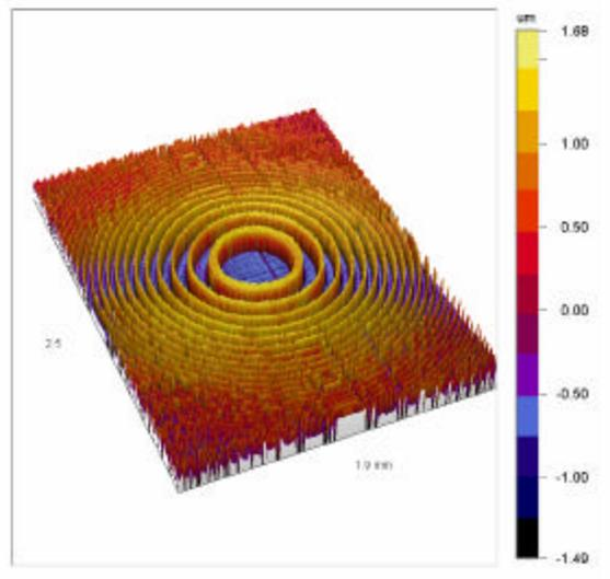
Grayscale Zone plate in photoresist
