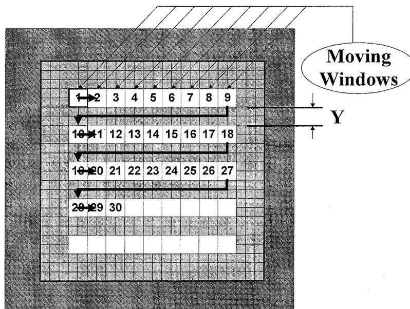
Fig. 2. Schematic diagram of moving windows on a LCD.
