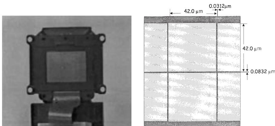
Fig. 1. Photograph and pixel structure of a LCD.
