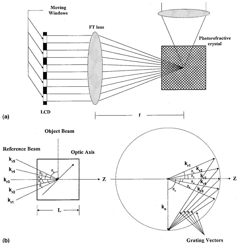
Fig. 3. Principle of angular multiplexing by moving windows (a) Interaction geometry in photorefractive material (b) Wave vector space description of holographic interaction.
