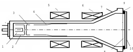
**Figure.1** Schematic diagram of M projection CRT
