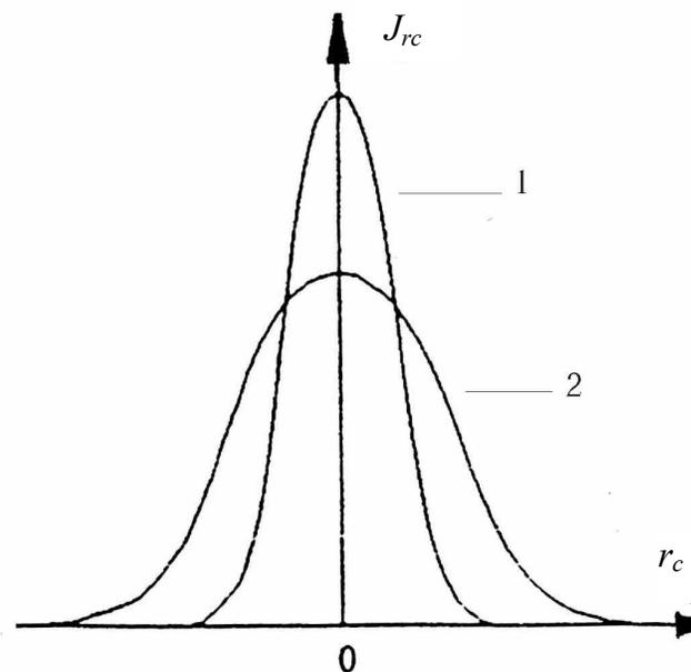
Figure.4 Current density distribution at crossover
