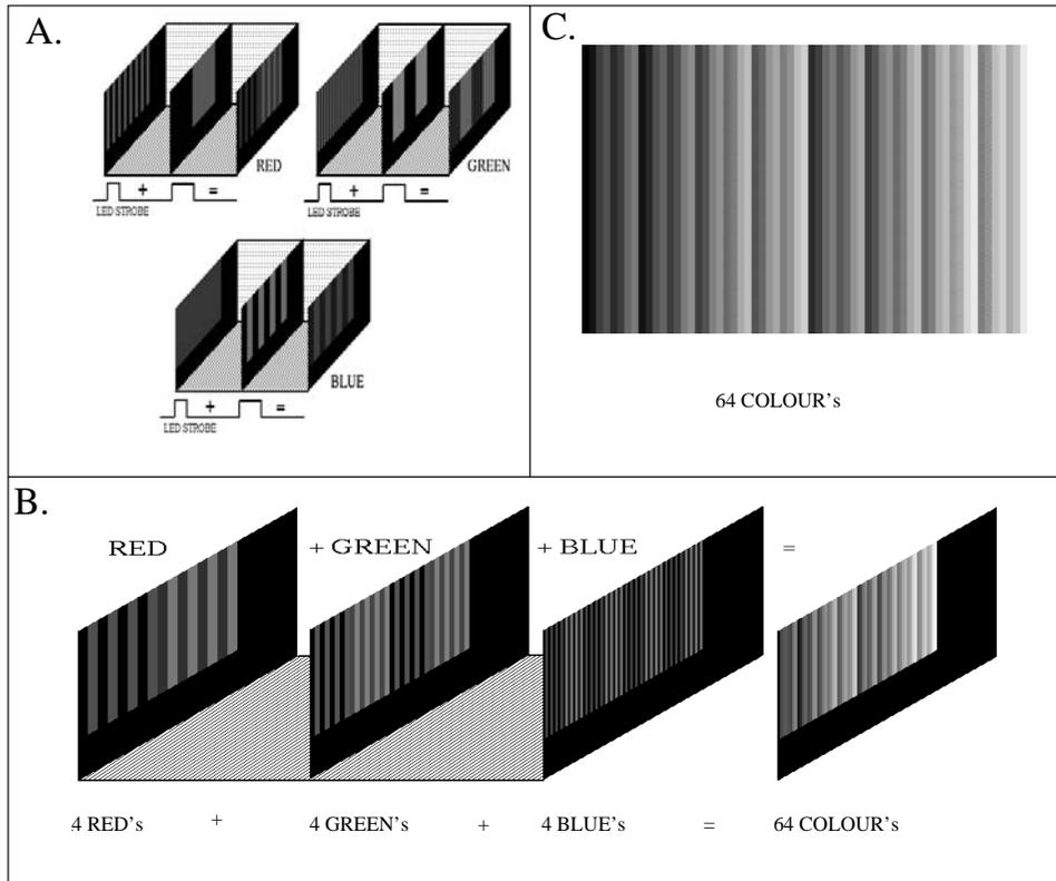
FIGURE 3 (A) 2 Monochrome binary frames, for each LED, produce 4 monochrome colour levels. (B) 4 RED's followed by 4 GREEN's and 4 BLUE's produce 64 different colours. (C) Simulated test image demonstrating 64 different colours. (Black and White reproduction)
