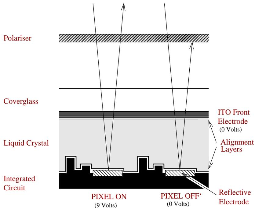
FIGURE 2 SLM Pixel Operation.
