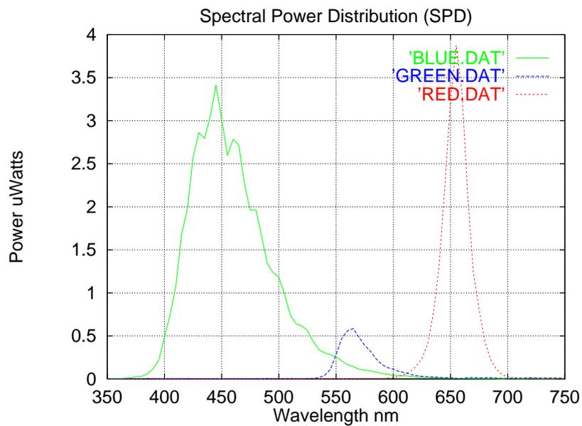
FIGURE 4 LED Spectral Power Distribution.
