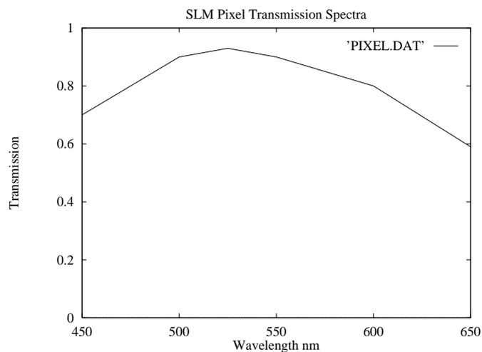
FIGURE 6 Transmission Spectra a single SLM pixel.
