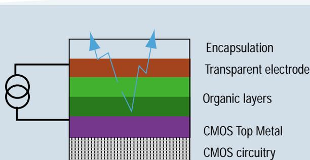
**Figure 1** In each pixel of an OLED microdisplay, the light-emitting organic layer is sandwiched between the CMOS circuitry and the top electrode, with additional organic layers such as 3,4-polyethylene-dioxythiophene polymer included to enhance performance .
