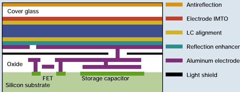
**Figure 2** In an LCoS display with an index-matched indium-tin-oxide transparent electrode and field-effect transistor, the liquid crystal acts as a spatial light modulator for illumination passing through the cover glass and reflecting off the bottom layer.
