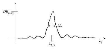
where  $\lambda_{2,0}$  is the central wavelength of the reflection spectrum, which we have seen above is determined by the exposing wavelength, shrinkage effects, and the angle of incidence. The maximum height of the curve, or  $DE_{\text{max}}$ , and the width of the reflection spectrum at its half-height points,  $\Delta\lambda_2$ , are what we are about to discuss. We have to
