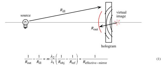
Note that all optical radii (and the mirror radius) are positive in the example diagrammed alongside. The value of m depends on which side of the hologram is being illuminated; m = +1 if the illumination is coming from the same side as the reference beam—there is no other diffracted order if the hologram is reasonably thick. However, the physical
