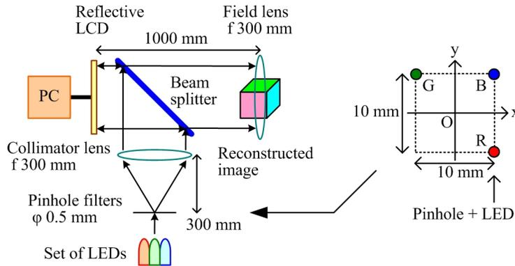
Fig. 6. Experimental setup for the color-reconstruction method presented here.
