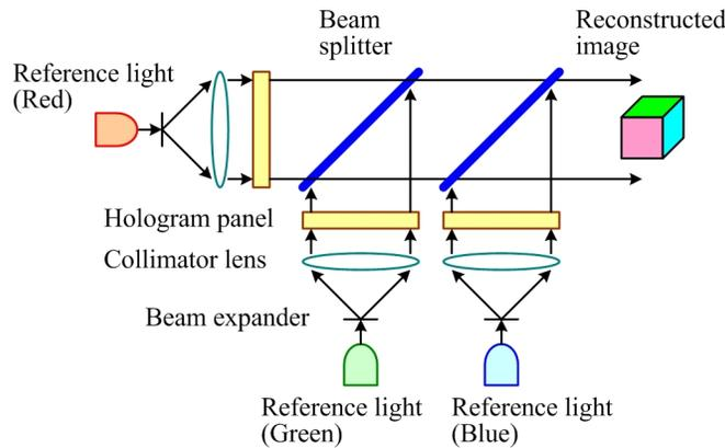
Fig. 1. Color electroholography setup: three hologram panels combined with three colored reference lights.
