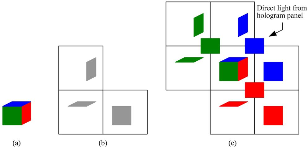
Fig. 5. (a) Cube with three colors, (b) separation of the color components, and (c) reconstruction by RGB reference lights.
