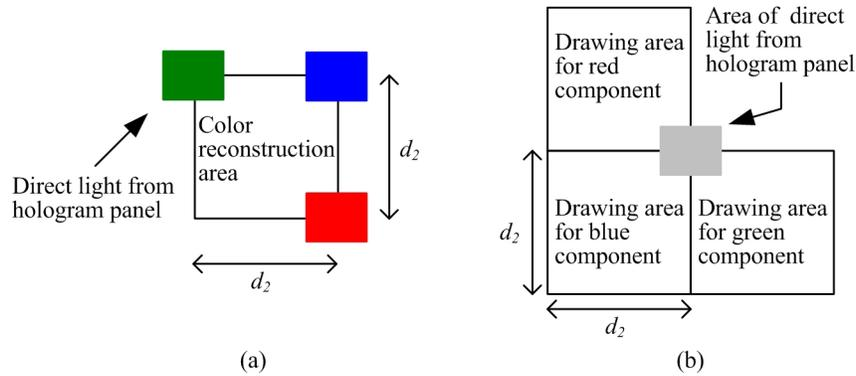
Fig. 4. (a) Color reconstruction of the area where a reconstructed image is focused and (b) areas of a three-dimensional object redrawn according to RGB color components.
