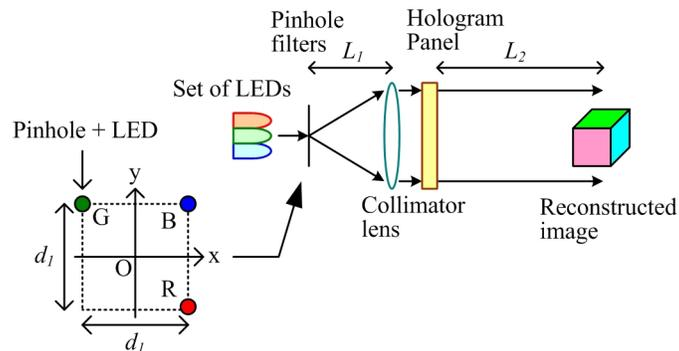
Fig. 3. Color electroholography setup for our proposed method. The reference light system is shown at the left.
