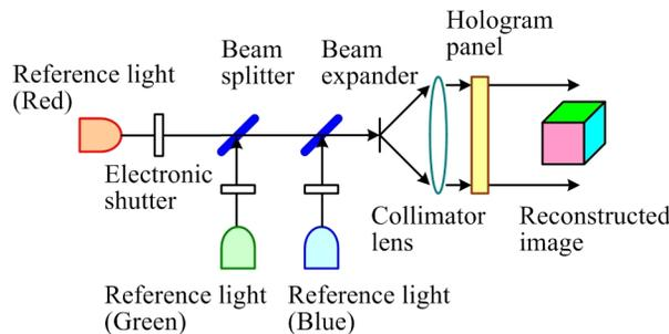
Fig. 2. Color electroholography by time-division multiplexing with one hologram panel.
