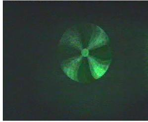
Figure 3. (1.74 Mb) Video presenting a rotating 2D propeller recorded in the Fourier transform recording setup (Figure 1b). The reconstruction speed is variable so stroboscopic effects are observed.
