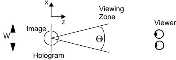
For a hologram located in the image plane (i.e., an *image-plane* hologram), the diffraction angle is equal to the viewing angle. (The image plane is the plane in the middle of the image volume.) Therefore, the image-plane requirement on sample count is determined by the size of the viewing zone. For a hololine of width  $W$ , the sample count becomes:
