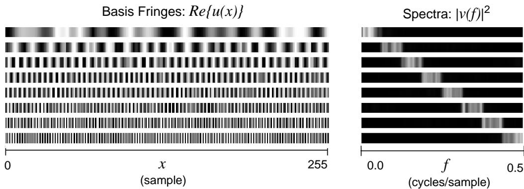
At its right is its spectrum. Included are an additional seven basis fringes, each with a spectrum that is rectangular with width  $\Delta_f=0.5/8=0.0625$ , each non-zero in the range  $[i\Delta_f,(i+1)\Delta_f]$  for  $i=[0,7]$ . These basis fringes evenly divide the spectrum into eight equal parts. Such a set of basis fringes was used to perform hogel-vector decoding for
