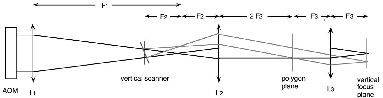
Figure 3. Vertical scanning optics. L<sub>1</sub> and L<sub>2</sub> are cylindrical lenses.
