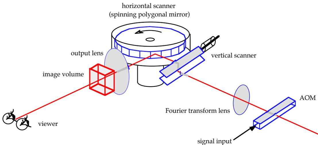
Figure 1.1 Electro-optical section of the MIT holographic display.
