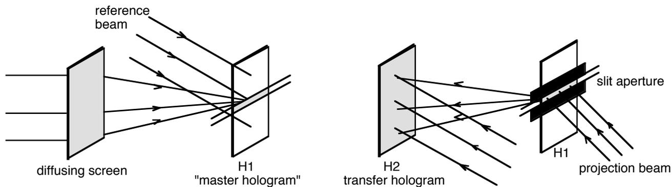
Figure 6. HOE master recording (left) and transfer (right)
