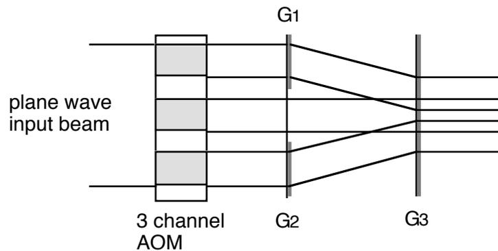
Figure 4. Holographic beam multiplexer
