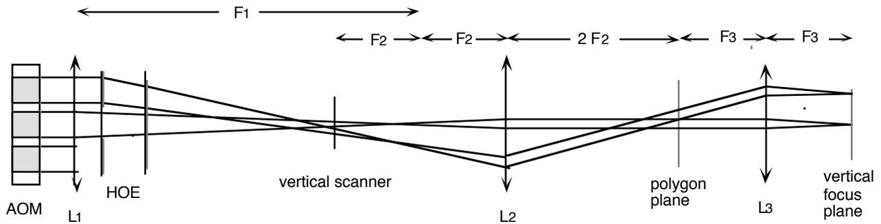
Figure 5. Vertical scanning using a three channel AOM
