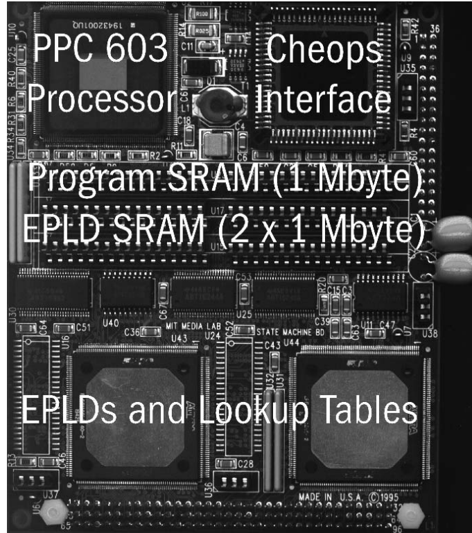
Figure 4: The State Machine stream processor, 75% of actual size.
