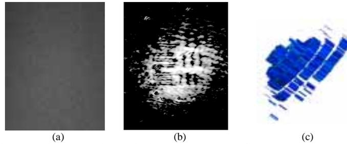
Fig. 5: (a) Direct "image" through 10 MFP (double pass) of scattering media. Holographic reconstruction of (b) USAF test chart through 13 MFP showing 50  $\mu\text{m}$  bars; (c) 3-D test object showing 100  $\mu\text{m}$  depth resolution through 10 MFP (double pass).
