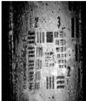
Fig. 2. (a) Holographic reconstruction of USAF test chart showing 50 \mu\text{m} bars.
