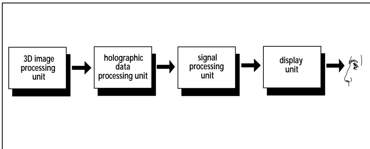
Fig. 2: Components of a holographic display system
