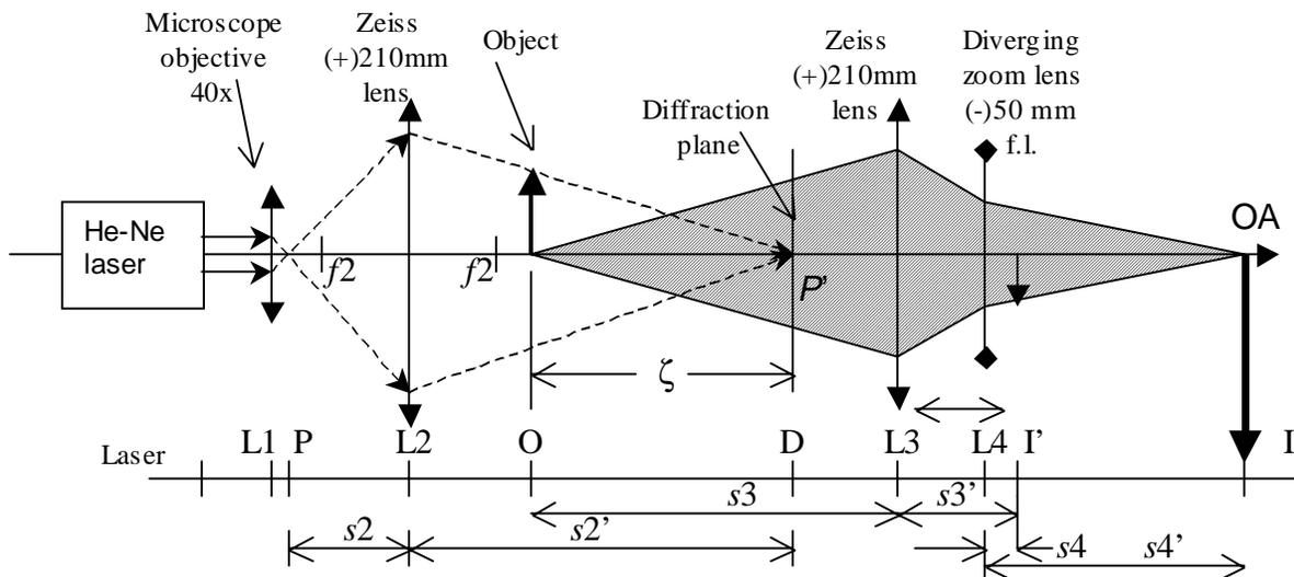
Figure 4.1. Converging beam Fourier optical analyzer.
