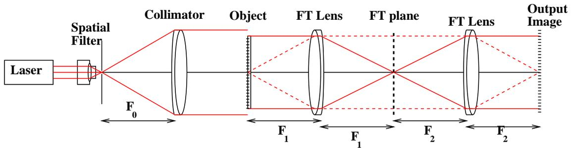
Figure 1: 4F optical system for spatial filtering
