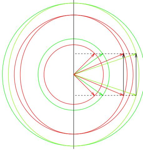
1. When a volume grating is written with green light from an Argon laser at a wavelength of 5145 Angstroms and read out with red light from a HeNe laser at 6328 Angstroms, the angle of the red beam must be adjusted for optimal Bragg matching. When we use  $\pm 10$  degrees for the two Argon writing beams, what should the angle of incidence be for the HeNe beam in order to obtain optimal Bragg matching?
