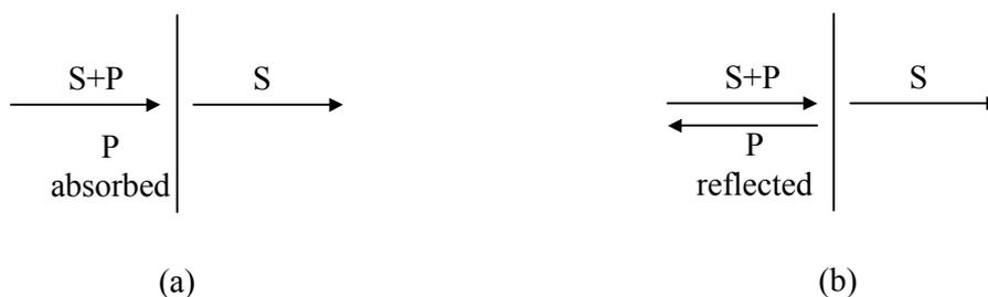
**Figure 5.4 : Absorbent (a) and reflective (b) sheet polarizers**
