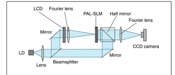
Figure 10: Analog optical computer structure
