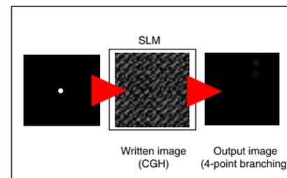
Figure 9: Concept view of optical interconnection
