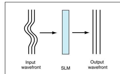
Figure 8: Wavefront compensation
