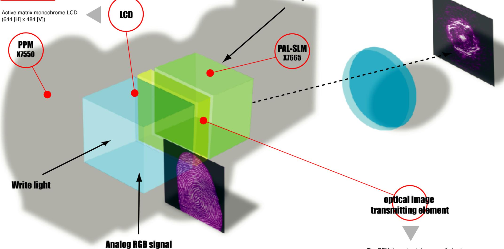
The PPM, in contrast, has an optimized coupling optics and a non-pixel structure of the PAL-SLM that does not transfer the pixel structure of the LCD into the PAL-SLM.
