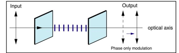
Figure 1: b) Parallel aligned nematic (PAL-SLM)
