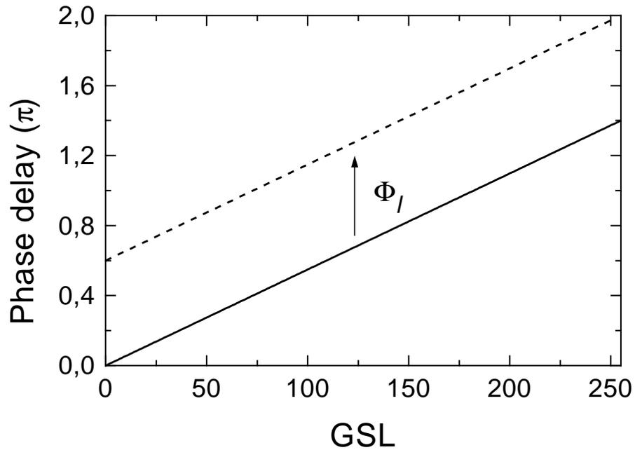
Fig. 3. Phase modulation characteristics of a mismatched SLM in the linear approximation. solid line shows the phase mismatching, i.e., the lower phase interval ( $0 - 1.4\pi$ ) is covered. Thus, the filter information contained in the interval ( $1.4\pi - 2.0\pi$ ) is lost.
