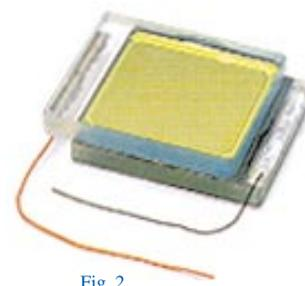
Fig. 2 Exterior of the PAL-SLM
