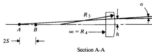
Figure 8 The toroidal lens designed for minimum ray deviation for all scan angles.
