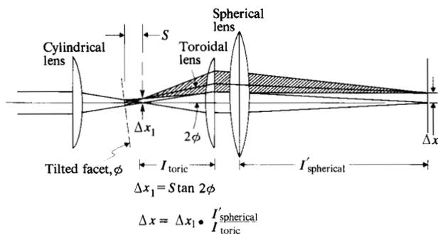
Figure 6 Scan line deflection due to sag  $S$ .
