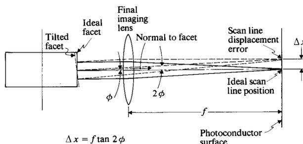
Figure 4 The scan line displacement error typical of rotating polygonal mirror scanners.
