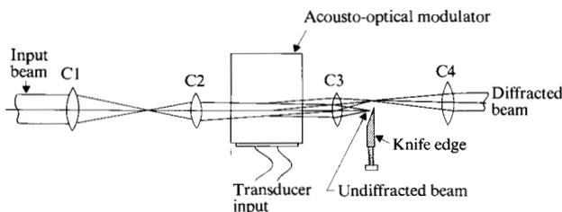
Figure 3 Detailed configuration of the compressor, modulator and beam expander. The beam is compressed by C1 and C2 and expanded by C3 and C4.
