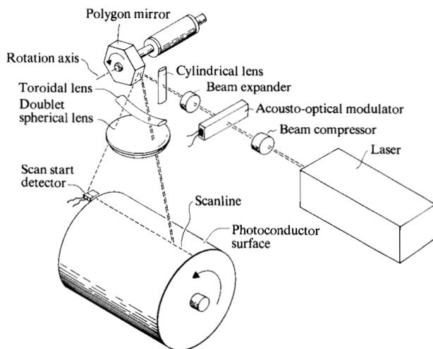
Figure 2 Laser subsystem, showing the polygonal mirror and scanning method.
