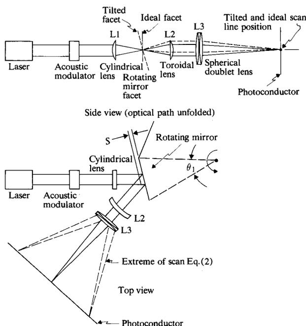
Figure 5 Cylindrical/toroidal lens correction technique.
