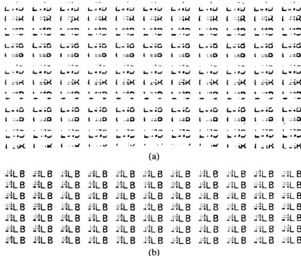
Figure 7 Print examples. (a) Without correcting optics. (b) With correcting optics.
